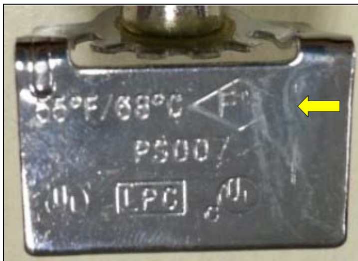
Figure 11 – Markings on the counterfeit horizontal sidewall (photo courtesy of UL, LLC)
