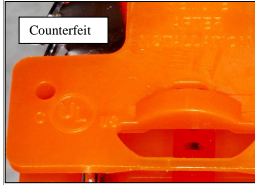
Figure 3 – Counterfeit shipping guard showing the UL Listed marking
