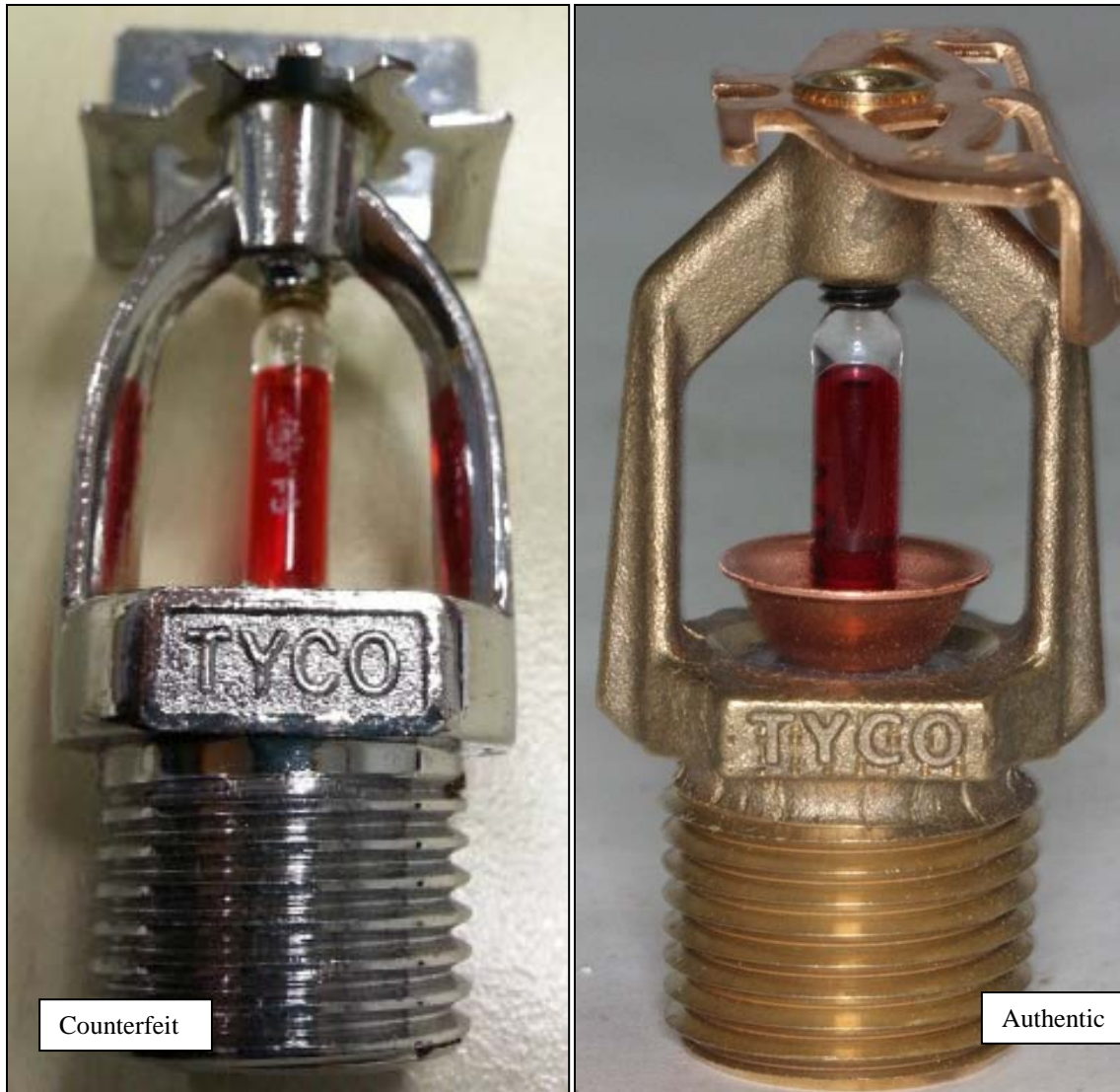
Figure 10 - Profile view of counterfeit horizontal sidewall sprinkler (left, photo courtesy of UL LLC) and an authentic Tyco TY3351 sprinkler (right)
