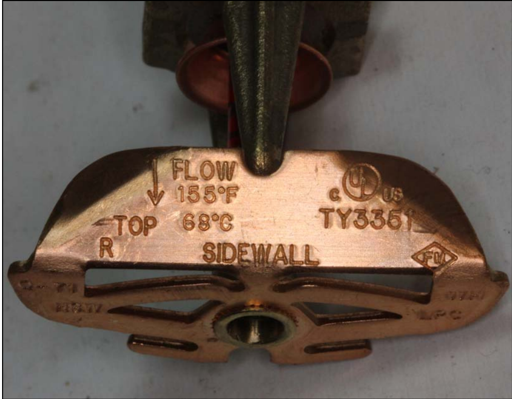
Figure 12 – Markings on an authentic Tyco TY3351 sprinkler
