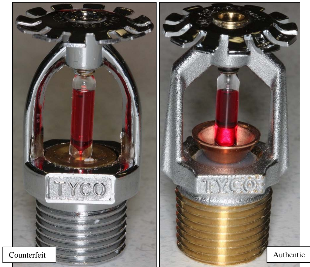
Figure 8 - Profile view of counterfeit pendent sprinkler (left) and an authentic Tyco TY3251 sprinkler (right)
