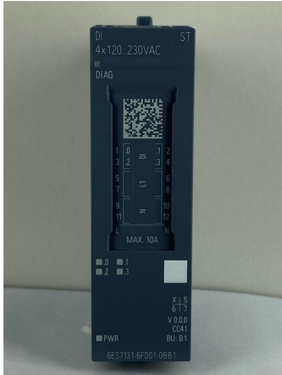
Figures 1 & 2 – Pictures of SIMATIC ET 200SP, Digital Input Module
