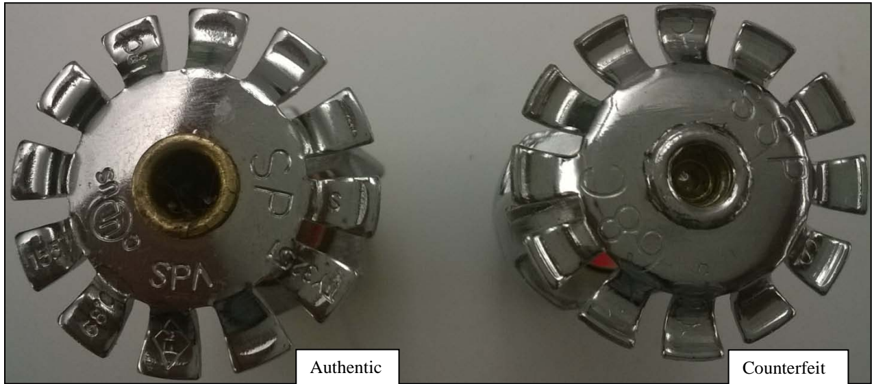
Figure 2 – Deflector and deflector markings on an authentic Tyco TY3251 sprinkler (left) and on the counterfeit sprinkler (right)
