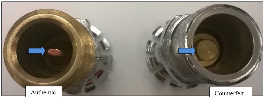
Figure 5 – Inlets of an authentic Tyco TY3251 sprinkler (left) and counterfeit sprinkler (right)
