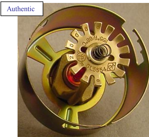
Figure 17. The photographs to the left show the authentic GL5654 sprinkler and the counterfeit sprinkler with similar attributes, identified as the model GL5681 sprinkler. The counterfeit sprinkler shares no similar parts with the authentic version. Globe Fire Sprinkler Corporation does not manufacture concealed sprinklers with chrome plated frames and deflectors. Chrome plating is intended for aesthetic purposes and is therefore not necessary on concealed models where the frame and deflector are hidden from view by the cover plate and would only add cost to the final product
