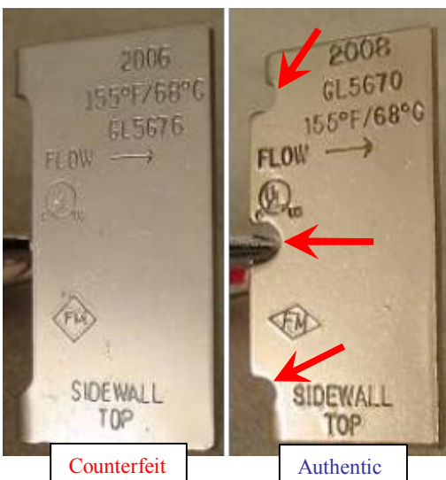
Figure 8. The deflectors of the counterfeit GL5676 (far left) and the authentic GL5670 (immediate left) are fairly similar in all but one place. The authentic GL5670 has three slots in the edge of the deflector towards the frame, shown by the three red arrows, while the counterfeit deflector has one wide slot spanning most of its width. The top and bottom of that same edge of the deflector is different on the authentic version as well.
