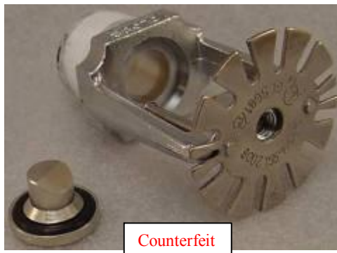
Figure 18. The photograph to the left shows the counterfeit sprinkler version with the escutcheon and heat sensitive element removed, and the orifice seal and cap assembly placed along side the frame assembly. The seal cap assembly was removed to determine the type of water seal employed in the counterfeit sprinkler. As shown in the photograph, the seal is an o-ring type, unlike the coated spring disc type seals used in all authentic Globe sprinklers. Also visible is one of the deflector pins, used for the drop down deflector, which is meant to slide downward after activation of the cover plate. Globe does not use a drop down deflector design in any of their authentic concealed pendent type sprinklers.
