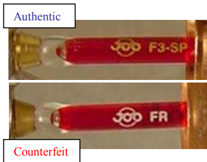
Figure 6. The photographs to the left show enlarged views of the thermal activation elements found in the authentic sprinkler (top) and counterfeit (bottom) sprinklers. Note the authentic Globe sprinklers utilize the Job model F3-SP bulb while the counterfeit sprinkler uses a Job model FR bulb. It is important to note Globe is Approved to use both the Job model F3 (with white bulb lettering) as well as the model F3-SP (with gold lettering) in the GL5601 but is not Approved to use the Job model FR bulb. Any Globe GL5601 sprinkler with the FR marking on the bulb should not be considered an authentic Globe product.
