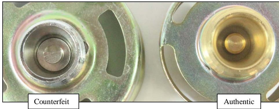
Figure 4. Differences in appearance of the water side of the orifice caps and seals of one of the counterfeit sprinklers (left) and an authentic Globe sprinkler (right).
