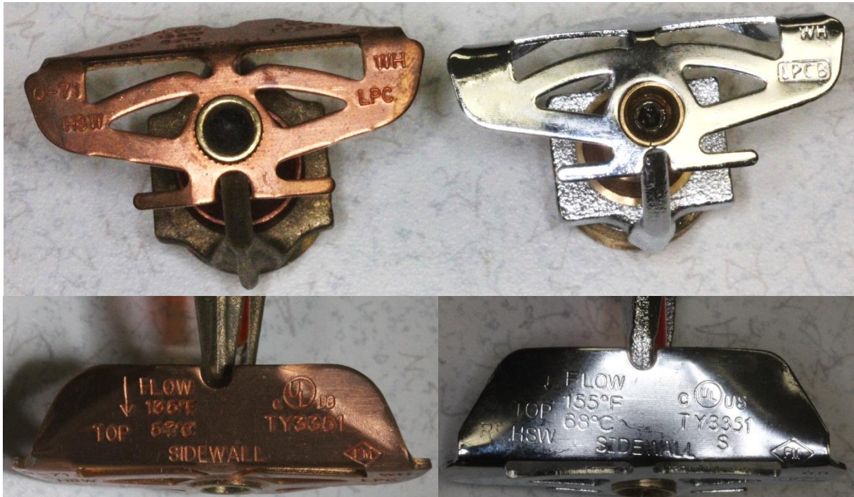
Figure 3. Authentic TY3351 deflector (left) and counterfeit deflector (right). The markings are similar, including the appearance and position FM Approvals mark.
