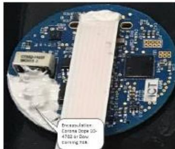
Fig-1: Board with correct encapsulation
