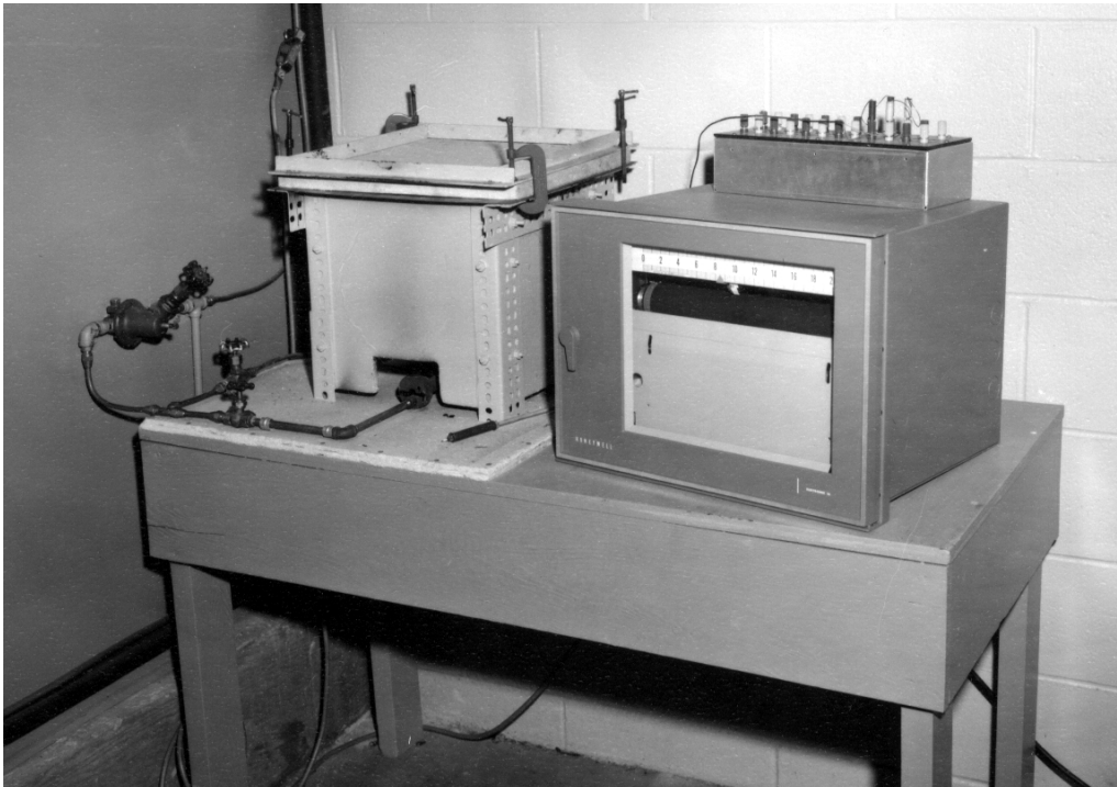
Figure G-1. Heat Damage Test Apparatus
